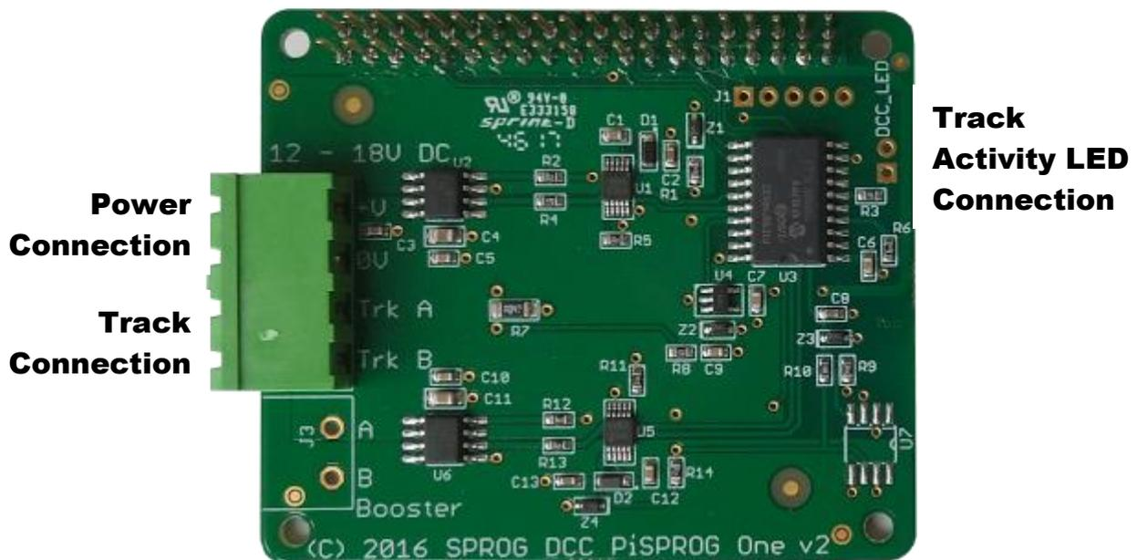
Pi-SPROG 3 is a firmware upgrade for Pi-SPROG One hardware, hence the “PiSPROG One v2” legend on the circuit board.
